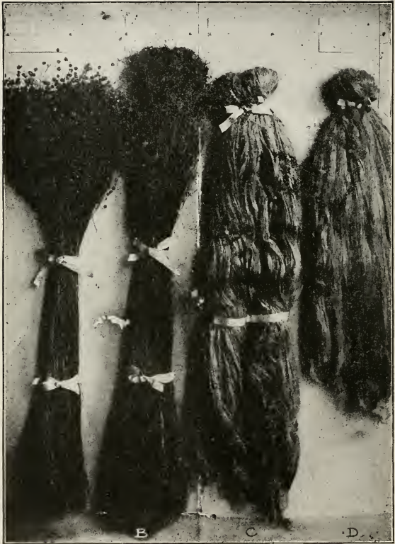
FLAX A, Unthrashed Straw; B, Retted; C, Cleaned or Scutched; D, Hackled or Dressed. (Photograph of C. R. Dodge).
